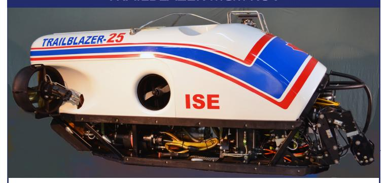
The ISE Trailblazer MCM ROV is a lightweight, highly manoeuvrable solution to mine detection, survey, recovery and disposal requirements. Developed by ISE specifically for MCM roles, the Trailblazer has successfully demonstrated its capabilities in Norway, Oman, Australia, the USA and Canada along with 4 other countries. Trailblazer is in current operational service with the Canadian Navy.
