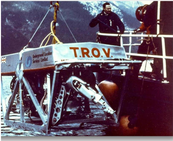
TROV (Tethered Remotely Operated Vehicle) One of the first ROV's developed by ISE in 1976
