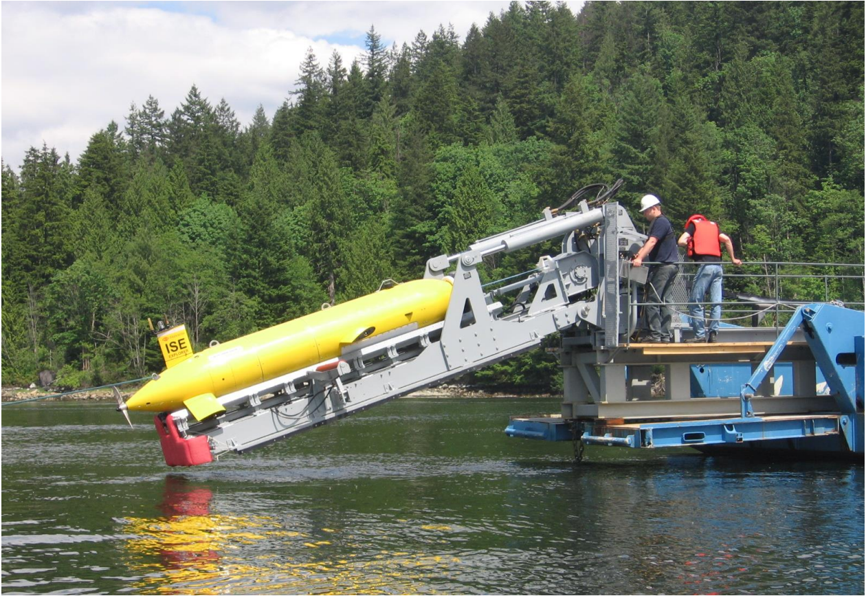
AUV with self-articulating ramp-based Launch and Recovery System (LARS)
